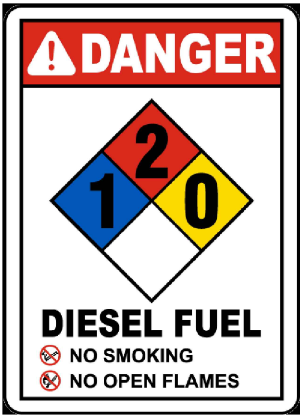
10"x14" MIN. NFPA DIESEL FUEL 1-2-0 DANGER SIGN (MYSAFETYSIGN.COM PN: M3348-AC OR EQUIVALENT)
